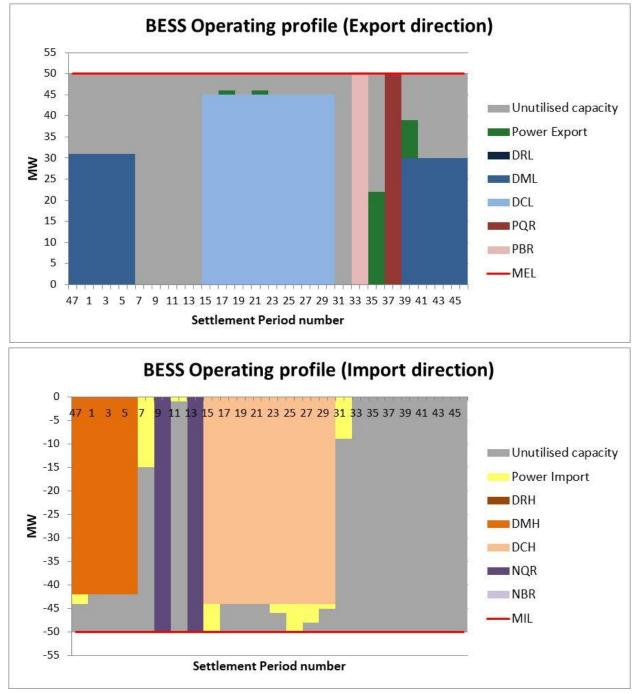
The optimised Balancing Reserve, Quick Reserve, Dynamic Frequency Response Service and power export and import levels in each Settlement Period for a 50MW / 50MWh BESS over a one day period. Sufficient headroom is maintained to ensure at least the minimum required level of Energy Recovery is possible following a period of response delivery.
